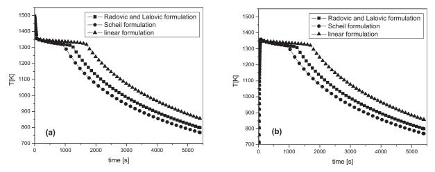
Figure 6. Thermal profiles for the mold/metal system concerning condition 7, 8 and 9 of Table 1. (a) Inside of the cast-point 1, (b) Inside of the mold-point 2.
