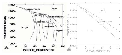
Figure 2. Phase diagram of Cu-5 wt %Zn alloy [18].
