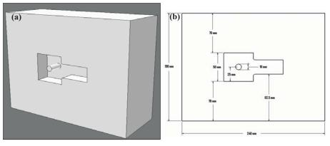
Figure 1. The cast part and mold in 3-D and 2-D.
