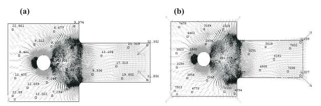
Figure 4. (a) Thermal gradient (K/m) in vectorial form and (b) Heat flux  $(W/m^2)$  in vectorial form (Line 9 of Table 1).
