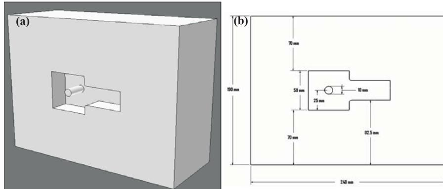
Figure 1. The cast part and mold in 3-D and 2-D.
