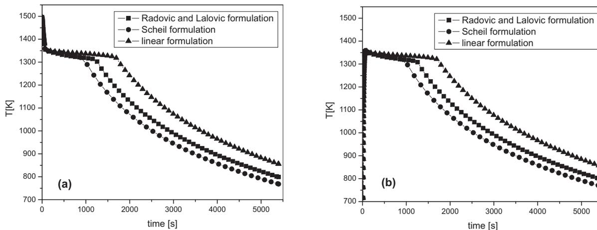
Figure 6. Thermal profiles for the mold/metal system concerning condition 7, 8 and 9 of Table 1. (a) Inside of the cast-point 1, (b) Inside of the mold-point 2.
