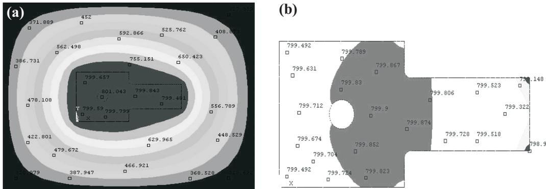
Figure 3. Temperature distribution in the (a) sand mold system, (b) cast metal (Line 9 of Table 1).
