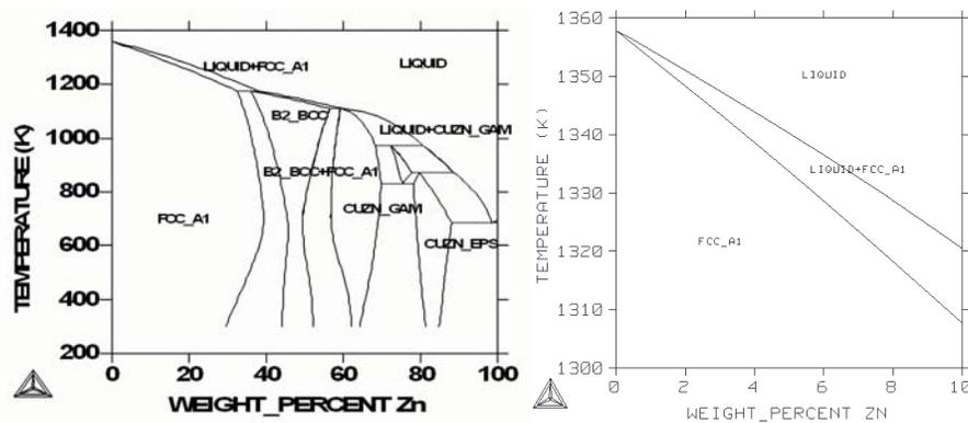
Figure 2. Phase diagram of Cu-5 wt %Zn alloy [18].
