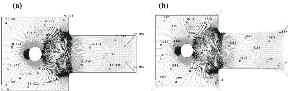
Figure 4. (a) Thermal gradient (K/m) in vectorial form and (b) Heat flux (W/m<sup>2</sup>) in vectorial form (Line 9 of Table 1).
