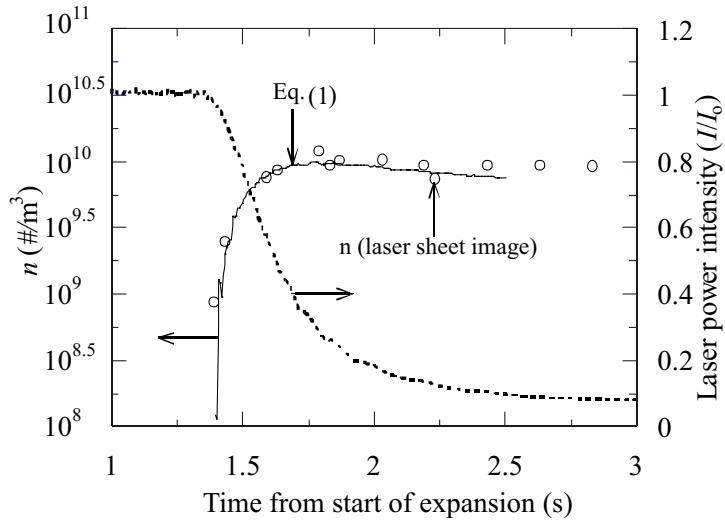
Figure 5. Variation with time of laser power attenuation and droplet number density.
