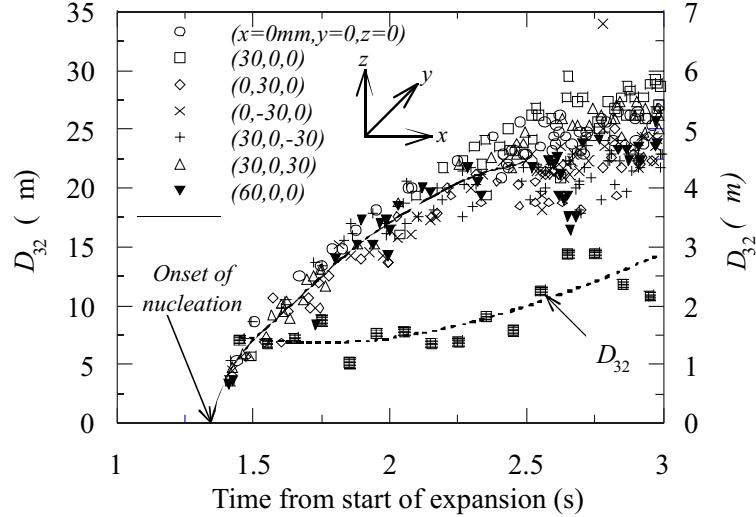
Figure 4. Droplet size variation with time and space. Conditions are the same as in Figure 3.
