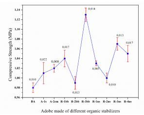
Figure 3. Standard deviation of adobe compressive strength values for each combination.
