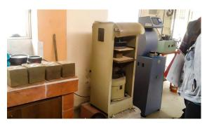
Figure 1. Standardized adobe samples for the test in the compression machine.
