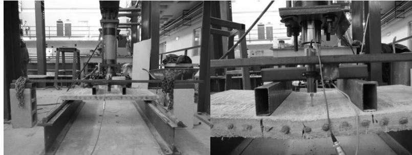
Figure 3. Arrangement for the flexure test of the fiber-reinforced panels.
