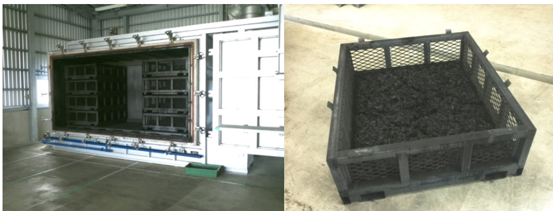
Figure 6. The used equipment and biochar. 1: the commercial scale charcoal kiln, 2: the charcoaled substrate.
