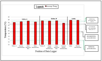
Figure 3 (a): Comparison of Average 40 Days Temperature with ASHRAE and UNI 10829/99
