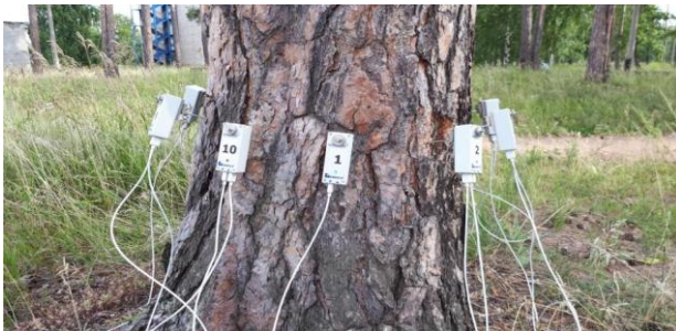
Figure 1 – The arrangement of the Arbotom® sensors on the tree no. 7.
