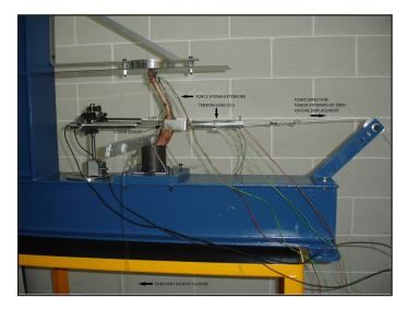
FIGURE 1. TESTING BENCH WITH SPECIMEN, MUSCULA-TURE SIMULATORS, MEASURING DEVICES AND APPLIED FORCE SYSTEM
